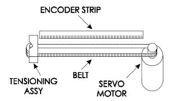
Figure 2-3. Carrier Axis Drive.
